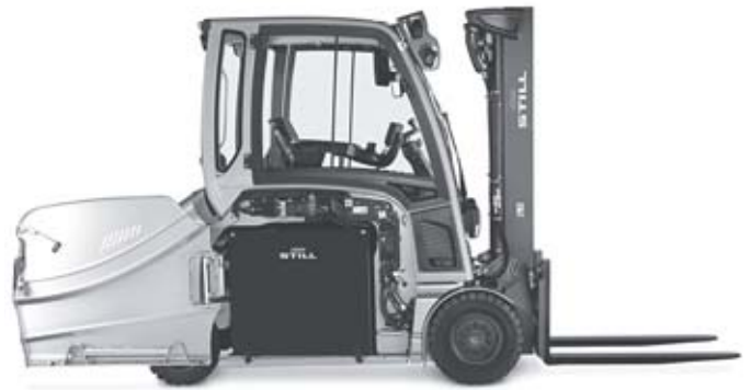
Optimum availability due to fast and safe battery change
