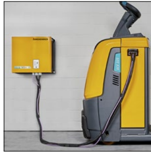
Lateral comfort charging plug for lithium-ion batteries (optional)
