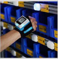
**EASY PAIRING** - the LIGHT TAG and the corresponding storage location are scanned and finally paired
