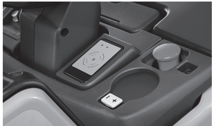
A variety of access options and a stand-on platform cushioning that can be adjusted by rocker switch (+/-) 3
